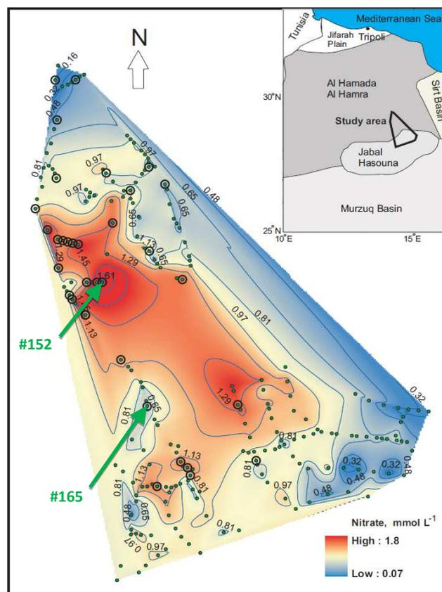
**Figure 1.** Sampling sites ( $\circ$ ;  $n = 28$ ) and distribution of  $\text{NO}_3^-$  in paleo-groundwater from Hasouna, Libya. Isolines are obtained from a total of 57  $\text{NO}_3^-$  analyses of paleo-groundwater from wells ( $\bullet$ ).
