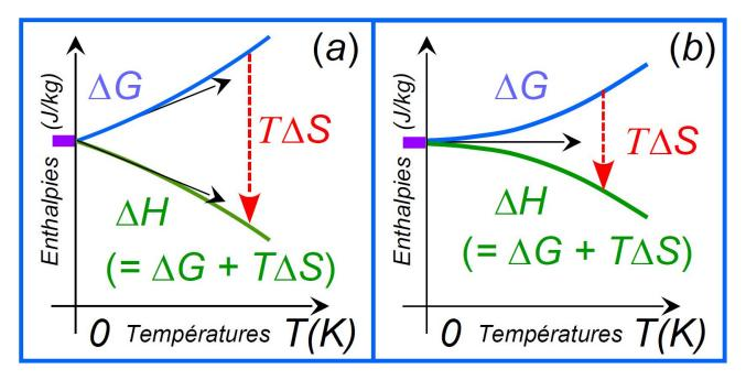
Figure 2: Graphical translation of the Nernst's theorem as expressed in his articles of 1906, 1907, 1910, but with modern notations. The curves for the change in free enthalpy  $\Delta G$  and in enthalpy  $\Delta H$  are plotted in ordinate as a function of the absolute temperature on the abscissa.
