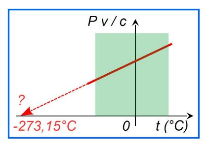
Figure 1: We draw here the quantity "Pv/c" given by the equation (1) as a function of the temperature "t" in Celsius. The usual range of atmospheric temperatures is drawn in green. The result is of the form "(t+a)". It is therefore a straight line that can be prolonged (in dashed lines) up to the ordinate "Pv/c = 0", where the temperature was "-a = -267" degrees after Gay-Lussac (1802), -273 degrees after Thomson (1848), and -273.15 degrees in the modern Kelvin scale.
