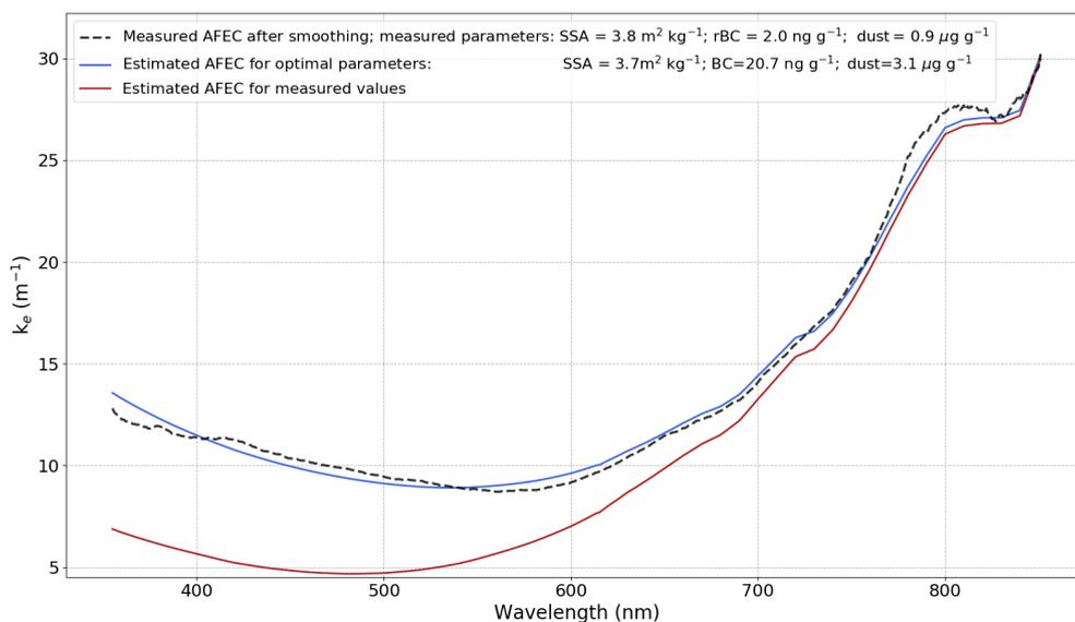
**Figure 14.** AFEC computation on a ZOI containing liquid water (between 15 and 18 cm on the SOLEXS profile 002 measured on 28 March 2017). The measured AFEC after filtering (black dotted line) is compared to the AFEC modelled using optimal parameters (blue curve) and to the AFEC modelled with measured values (red curves).
