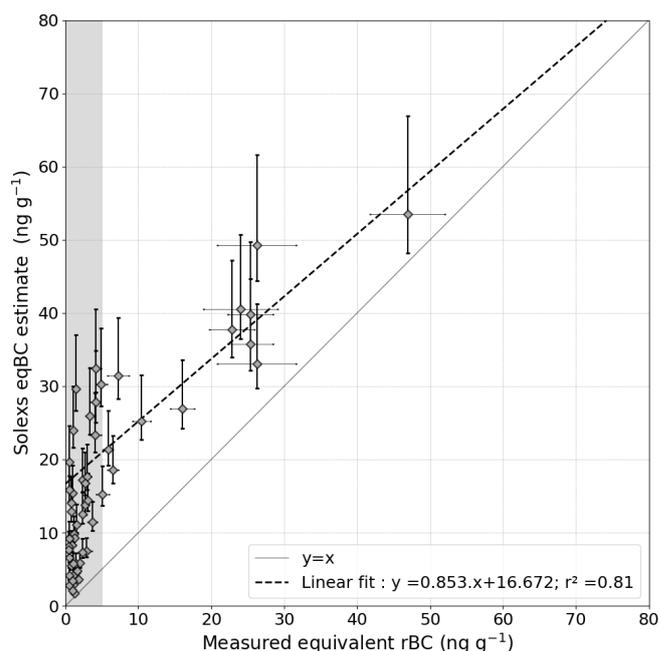
**Figure 11.** Comparison between measured and estimated eqBC concentrations for all the ZOIs with concomitant LAP measurement. The grey shading corresponds to the zone below the sensitivity limit of our method (i.e.  $5 \text{ ng g}^{-1}$ ). Error bars show how uncertainties on the enhancement parameter of ice B affect the LAP retrieval algorithm.
