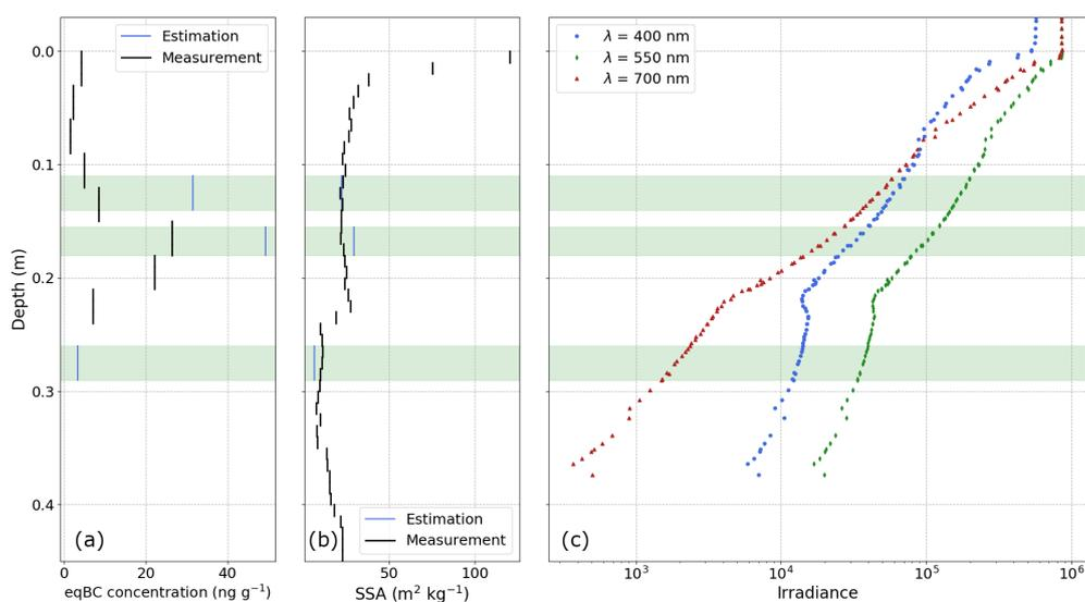
**Figure 6.** Comparison between snow pit measurements and estimated SSA and LAP concentrations for the SOLEXS profile 002 on 13 February 2018; green shading corresponds to the different ZOIs of the profile. **(a)** Vertical profile of eqBC concentration, measured (black) and estimated from AFEC optimisation on each ZOI (blue). **(b)** Vertical profiles of SSA, measured (black) and estimated from AFEC optimisation on each ZOI (blue). **(c)** SIP measurement from which AFEC has been derived.
