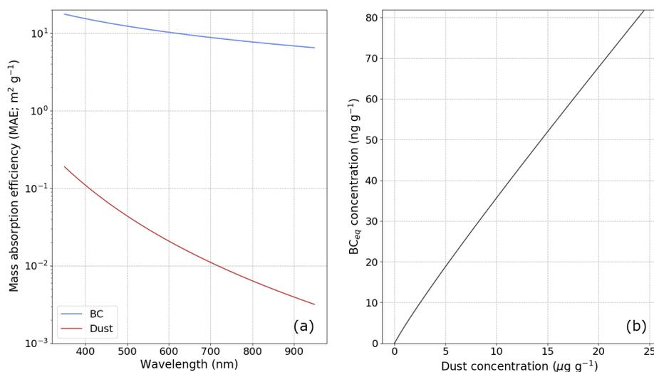
**Figure 1.** (a) Mass absorption efficiency (MAE) values of BC and dust used in the present study as a function of wavelength. (b) The eqBC concentration corresponding to a given dust concentration using these MAE values and the methods described in Sect. 3.1.
