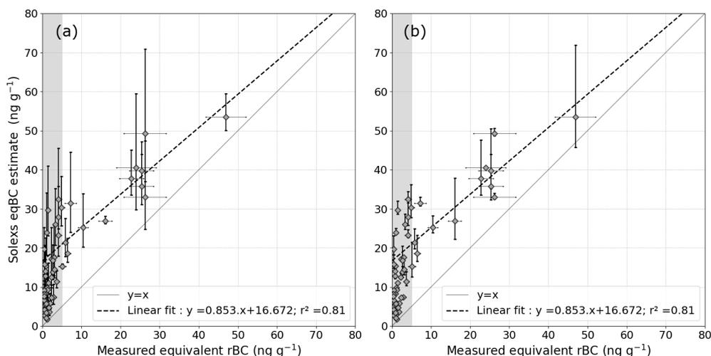
**Figure 9.** Comparison between measured and estimated eqBC concentrations for all the ZOIs with concomitant LAP measurements. The grey shading corresponds to the zone below the sensitivity limit of our method (i.e.  $5 \text{ ng g}^{-1}$ ). **(a)** Error bars show how uncertainties on BC MAE affect LAP estimates. **(b)** Error bars show how uncertainties on dust MAE affect LAP estimates.
