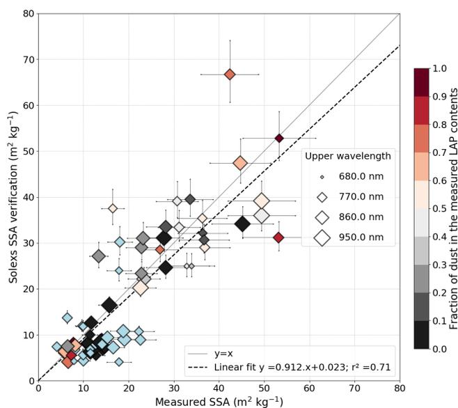
**Figure 10.** Comparison between measured and estimated SSA for all the ZOIs with concomitant SSA measurement. The colour of the symbols corresponds to the proportion of LAP absorption coming from dust, and sizes are related to the upper wavelength of the AFEC estimation. Symbols are blue when chemical measurements are not available.
