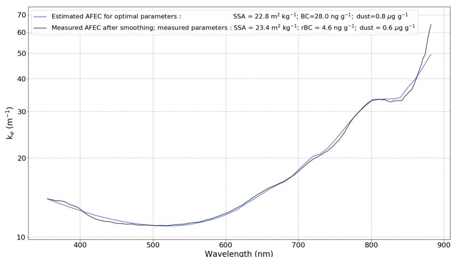
**Figure 5.** AFEC as a function of wavelength for the ZOIs between 11 and 14 cm on the SOLEXS profile 002 on 13 February 2018. Measured AFEC after convolution filtering (black curve) is compared to the estimated AFEC from Eq. (12) with optimal parameters (blue curve). Note that rBC is the measured refractory BC concentration by the SP<sup>2</sup> instrument.
