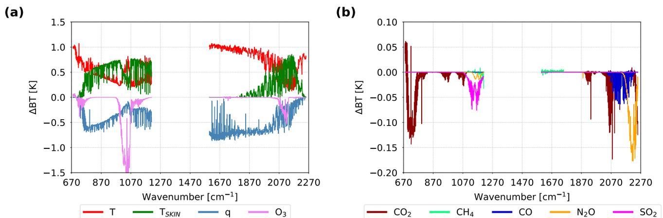
**Figure 2.** Sensitivity analysis of IRS brightness temperature to temperature, water vapour, ozone and skin temperature (a) and to carbon dioxide, methane, carbon monoxide, nitrous oxide and sulfur dioxide (b).
