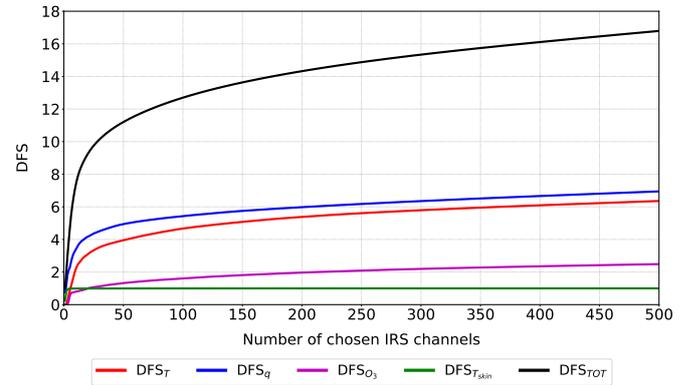
**Figure 10.** Evolution of mean DFS for temperature (red), humidity (blue), ozone (violet), skin temperature (green) and total (black) during the channel selection over the subset of 60 atmospheric profiles.
