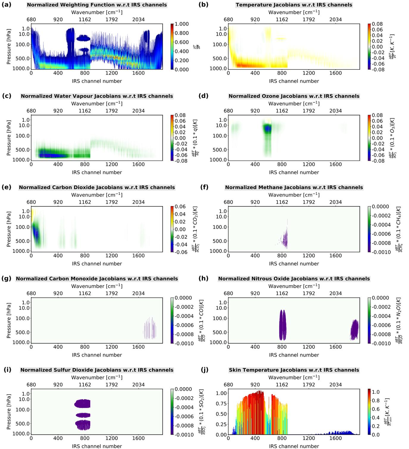
**Figure 3.** Mean of Normalized Weighting Function (a), Temperature Jacobians (b), Normalized Water Vapour (c), Ozone (d), Carbon Dioxide (e), Methane (f), Carbon Monoxide (g), Nitrous Oxide (h), Sulfur Dioxide (i) Jacobians with respect to pressure and Skin Temperature Jacobians (j) for IRS channels.
