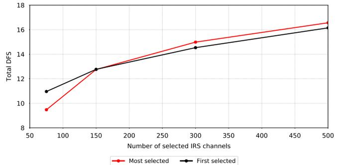
**Figure 13.** Evolution of the mean total DFS over 60 profiles as a function of the number of selected channels for the 75, 150, 300 and 500 first selected channels (in black) and the most selected channels (in red).
