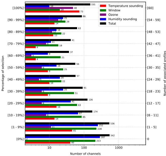
**Figure 11.** Percentage of the number of channels selected (up to 500 channels) on the subsets of 60 atmospheric profiles separated by spectral group and main application to temperature sounding (in red), humidity sounding (in blue), ozone (in violet), atmospheric window (in green) and total (in black) with respect to number of related profiles.
